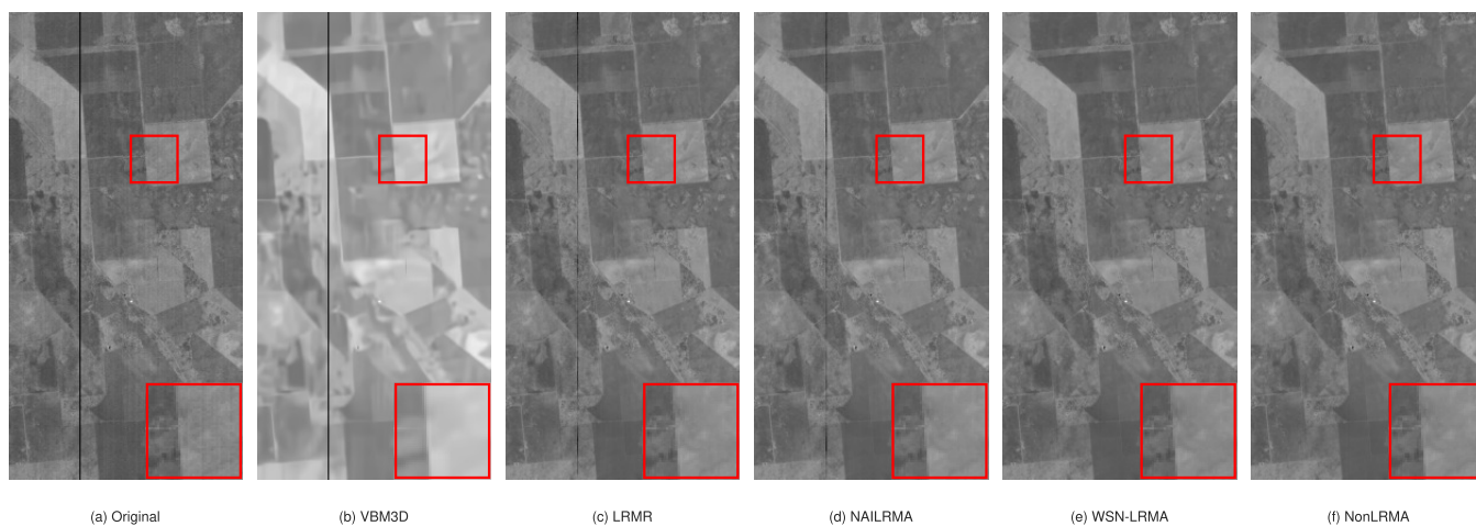
Fig. 15. Restoration results on Hyperion Australia data set: slight noise band. (a) Original image located at the 61st band. Resorted image obtained by (b) VBM3D, (c) LRMR, (d) NAILRMA, (e) WSN-LRMA, and (f) NonLRMA.
